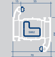
X862 - 'Z' TRANSOM/MULLION Reinforcement Options: S855 (Light) S862 (Stepped) S841 (Heavy)
